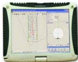
Flight Management System Touchscreen tablet PC in pilot's cabin for realtime position and course control
