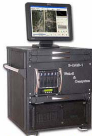
Control Computer Rack 2xOpteron64/PCI-X/RAM 4Gb RAID-3 2.0Tb/UltraSCSI-320/Touchscreen
