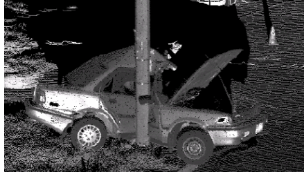
Crash scene evidence, featuring five scans merged into a single point cloud dataset
